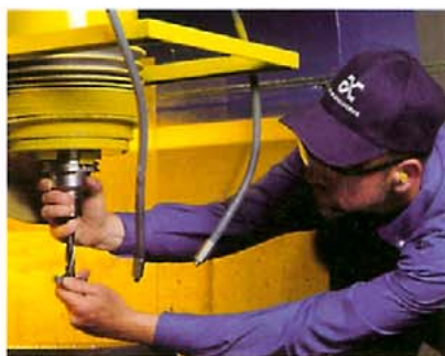
Changing tips on Qwik-Twist drill takes just seconds. Air-X-Changer uses one drill body for two different hole diameters.
