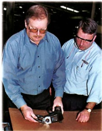
Dave Yambrosic (left) gages a finished part. US Manufacturing uses part tolerance and surface finish as indicators for indexing. With the new V-MAX inserts, tolerance and surface finish hold up at least three times longer, saving more than $200,000 a year in this high-volume operation.
