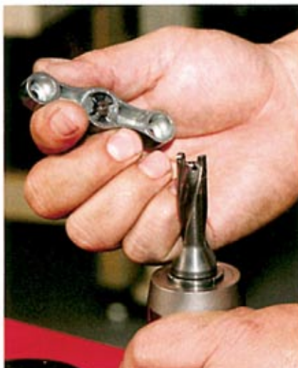
Changing the replaceable coated-carbide tip on the Qwik-Twist drill can be done in-house in just seconds.
