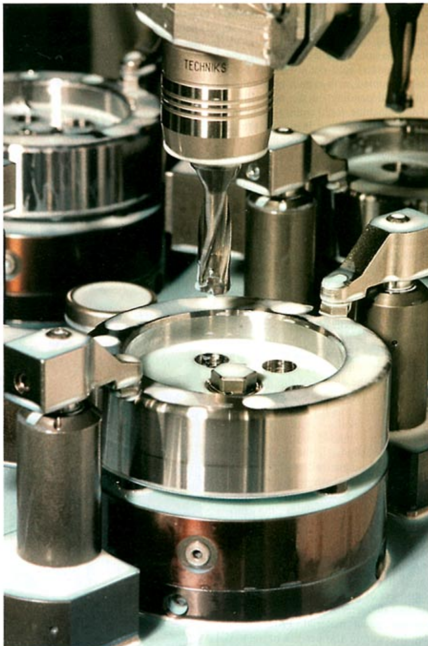
At Global Gear, Qwik-Twist replaceable point drills dramatically reduced drill inventories in production drilling of auto parts.
