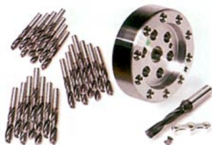
At Global Gear, a single Qwik-Twist drill (right) took the place of all the solid carbide drills shown on the left.
